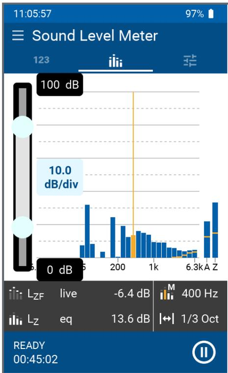
By long tapping on the X or Y axis, you can change the corresponding scale.
