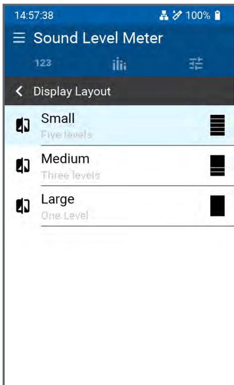
Three layout templates are available for the numeric level display.
