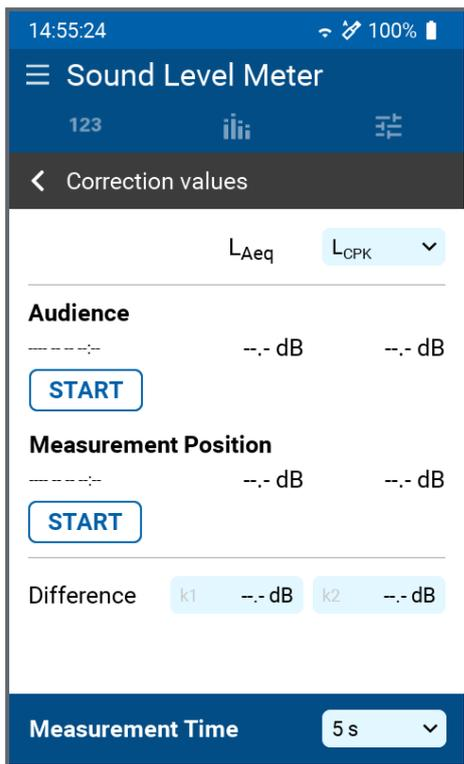
At live concerts, you often cannot place the meter directly at the loudest measurement location (**Audience**), but must place it at an alternate location (**Measure**). This leads to differences between the A- and C-weighted levels measured at the substitute location and those prevailing at the measurement location. You can determine or correct these differences by a simple measurement with the XL3.
