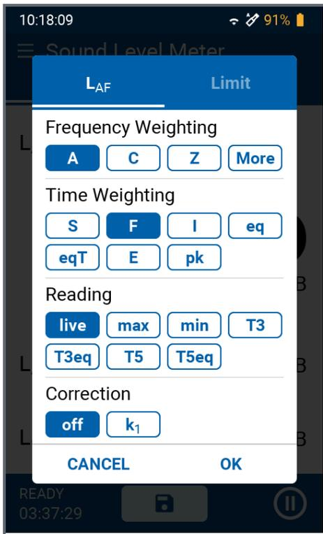
To display or change a specific level, tap on this level designation. This opens a menu where you can select the frequency weighting, the time weighting and any offset values for this level.
