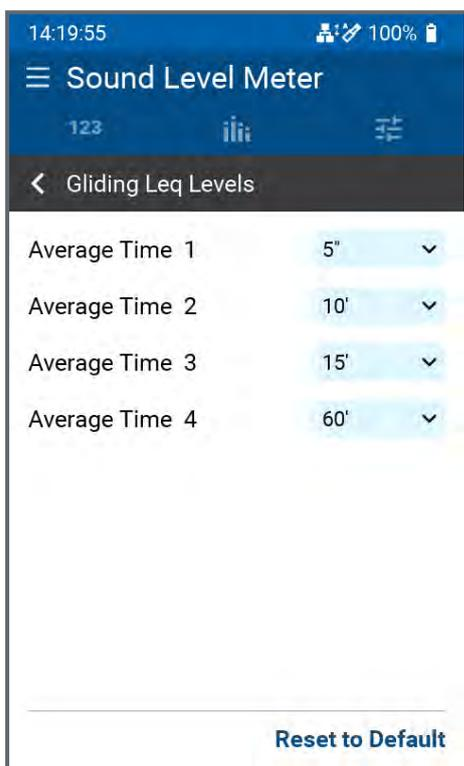
In addition to the mean value (Leq), which represents the entire measurement period from START to the observation time STOP, there are also moving averages Leqt, which calculate the mean value for a defined measurement period up to the observation time. The XL3 can calculate up to four moving averages in parallel to satisfy different national requirements.
