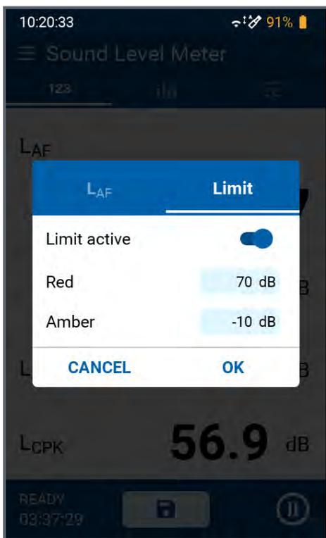
Under "Limit" you can activate and define a maximum limit ("Red") and an offset ("Orange Offset") for each individual level. As soon as the sound level exceeds the limit value, the display of the measured value changes to **red**. If the sound level in the "offset" range is directly below the limit, the display changes to **amber** (warning). Lower levels are displayed in normal **black**. Confirm the level input with OK on the on-screen keyboard.
