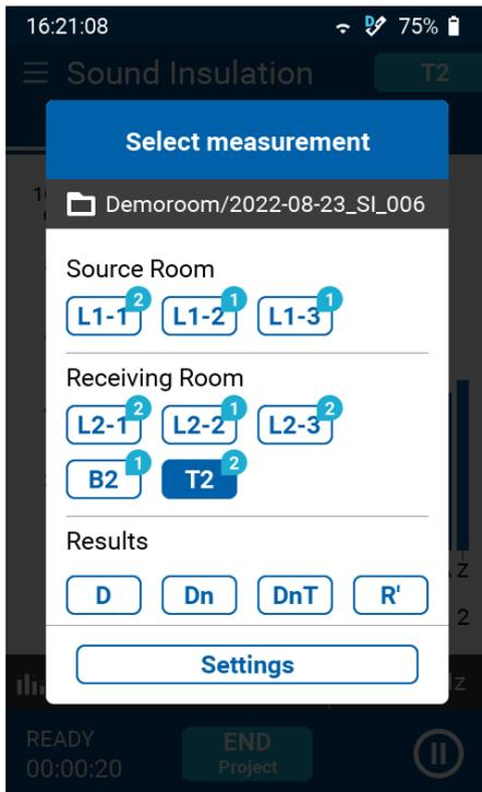
NOTE: At any time during an ongoing measurement series, you can view how many individual measurements have been performed in the transmitting or receiving room at the various positions of the sound source on the "Select measurement" page.
