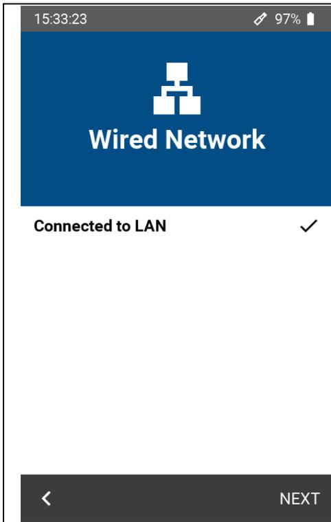
Alternatively, you may also connect the XL3 to a wired LAN network by plugging an Ethernet cable via adapter to the USB-C connector.
