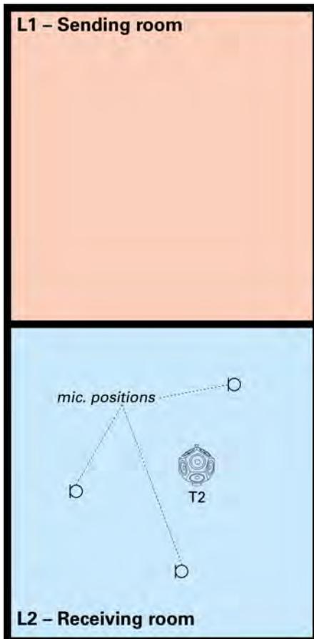
Now place the dodecahedron loudspeaker in the receiving room to determine the reverberation time  $T_2$ .
