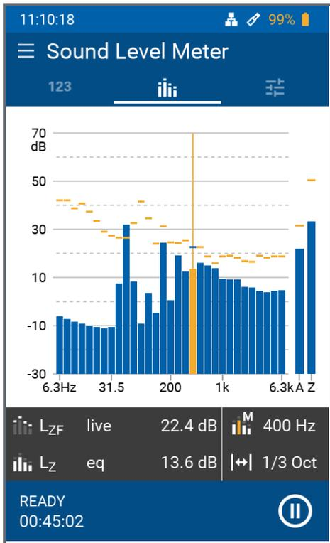
In the spectral display up to 2 spectra as well as the A- and Z-weighted broadband levels are displayed simultaneously.
