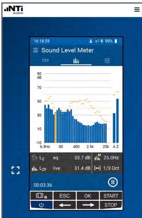
You can now control the device remotely with the mouse - just as if you were working directly on the device. If the screen of the web interface is touch-sensitive, you can also use this touch screen for the operation.
