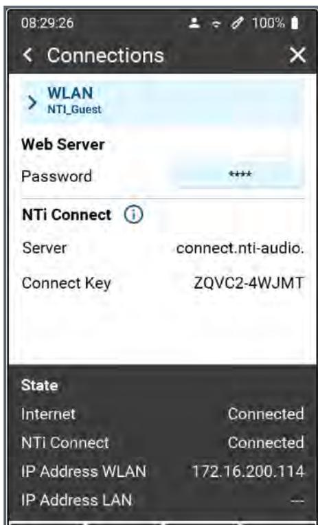
This setup shows the current status of the Wi-Fi connection and the assigned IP address of the device. The IP address is important for the connection with the web server. Under NTi Connect you may see the URL of the connection server and the unique connection key of your XL3. This key and the to be defined password are the required elements for a connection to the instrument via NTi Connect.
