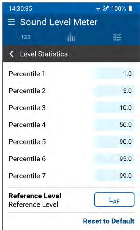
The instrument calculates up to 10 different percentile levels for broadband and spectral measurements. These data represent the statistical sound level distribution, and are typically used for environmental noise measurements. Here, for example, LAFxx% corresponds to a noise level exceeded during xx% of the measurement period. The 10 percentile sound levels are flexibly adjustable from 0.1% to 99.9%.
