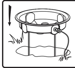
3. Dig a hole that is 15" wide and 5" deep. Place speaker base into the hole in the ground with the top rim of the base at ground level. Back-fill dirt into hole. For added security, cement security brackets into ground.
