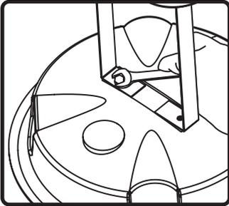
1. Attach inground/security brackets to speaker base using stainless-steel bolts.
