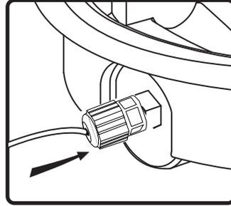
2. Field route Cat5 cable from the switch to each IPD-XT850, direct burial cable or use of conduit is required. The cable may need to be terminated after routing the cable through the compression fitting of the liquid-tight RJ45 coupling. Tighten fitting to seal.
