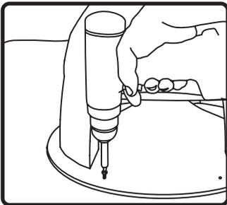
5. Set speaker enclosure on speaker base. Use tamper-resistant stainless-steel screws to attach speaker to base (driver tip and screws provided).
