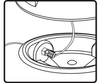
4. Plug Cat5 cables into coupling. No wire nuts needed. Tighten fitting to seal.
